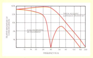
shown, the typical Koss system requires an average excursion of less than 15% of that required by the acoustic suspension system over a range of 2½ octaves in the low bass spectrum.
